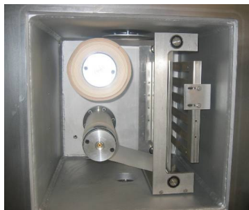
Fig. 2: Europlasma CD400 PLC with trays or roll cassette. LOW PRESSURE PLASMA ACTIVATION
